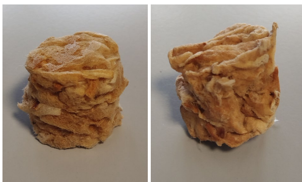
Figure 7. Effect of the binder on the samples: 10% concentration on the left, 80% on the right.
