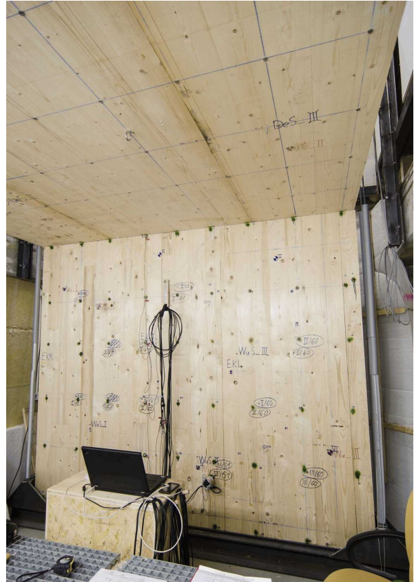
Figure 1. Bottom view of the junction mock-up.
