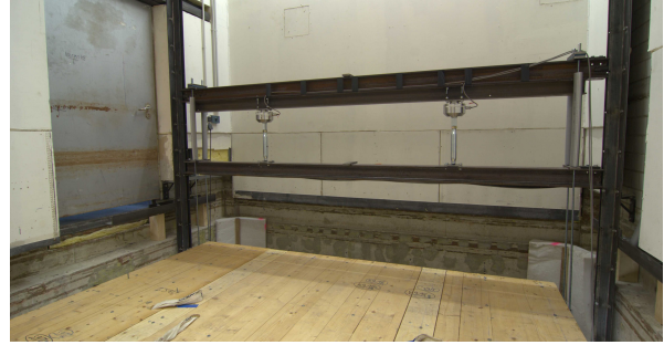
Figure 3. Top of the L-junction shown in the section drawing in Figure 2. Steel girders to apply a load on the junction. Between the two horizontal girders load cells are in place to measure the force.
