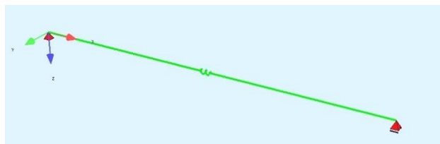
Figure 3. Single degree of freedom System (SDOF) calculation model
