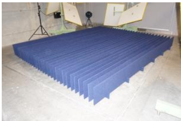
Figure 4. The baffle array with 100 mm spacing without a surrounding enclosure.
