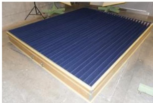
Figure 3. The baffle array with 100 mm spacing with a surrounding enclosure.
