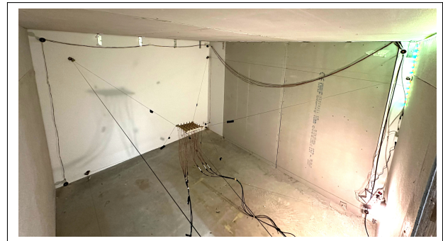
Figure 2. Photo of the cable robot showing the array connected by 8 cables to the attachment points at the room boundaries. Six loudspeakers used for microphone localisation are as well visible on the walls.
