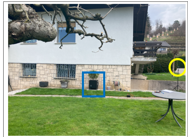
Figure 2. The 90^\circ incidence measurement setup with the loudspeaker (blue square) and the free field microphone (yellow circle).
