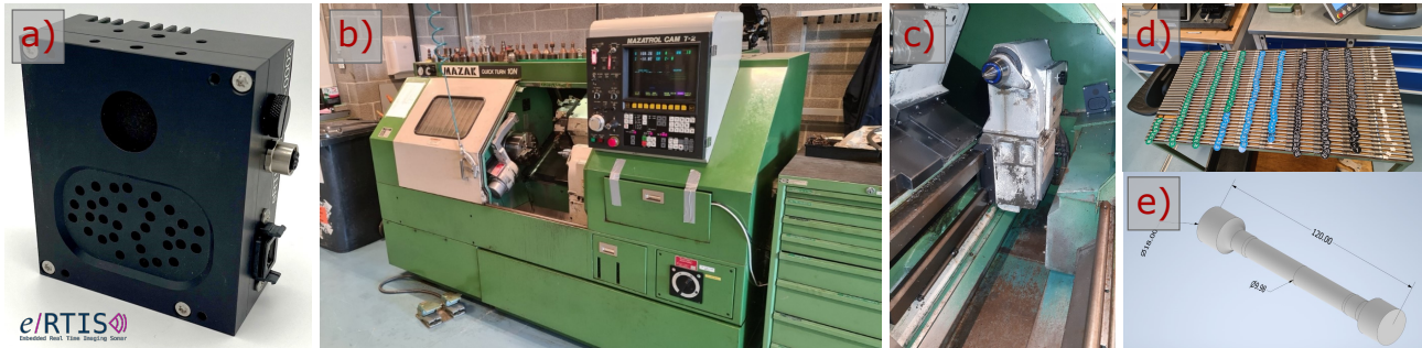
Figure 1. Overview of the hardware setup used in this paper. Panel a) shows the eRTIS sensor, an ultrasonic array sensor with 32 microphones arranged in a pseudorandom pattern. The sensor is waterproofed using a membrane material from the Acoustic Protective Material line manufactured by W. L. Gore and Associates. Panel b) shows the CNC lathe being used, a Mazak Quickturn 10N, using Iscar GRIP 3015Y grade IC808 inserts. Panel c) shows the inside eRTIS sensor mounted in the lathe. Panel d) shows the turned materials, and e) shows the model of the piece that has been turned during this experiment.
