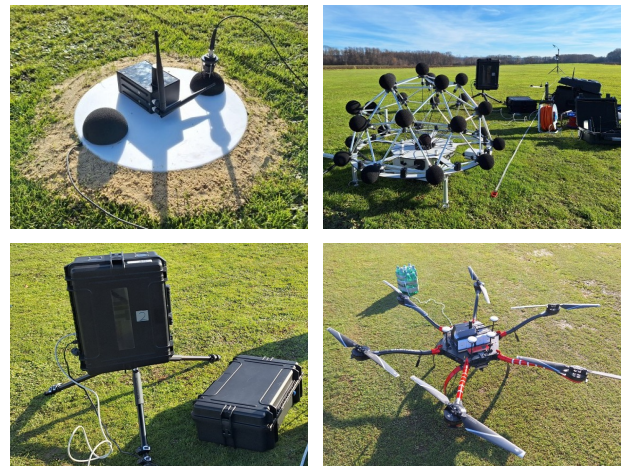
Figure 1: Measurement setup: SPL with GNSS for positioning (top left), ARR with windscreens (top right), CAM in case (bottom left), and a ViewCopter V6H with payload for MTOM (bottom right).
