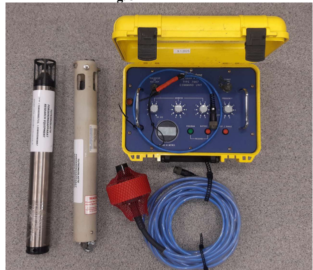
Figure 3. Hydrophone (530x60 mm, 2.6 kg with 12 A-batteries), acoustic releaser (AR, 490x64 mm, 1.8 kg with batteries), AR controller unit, and AR transmitter.
