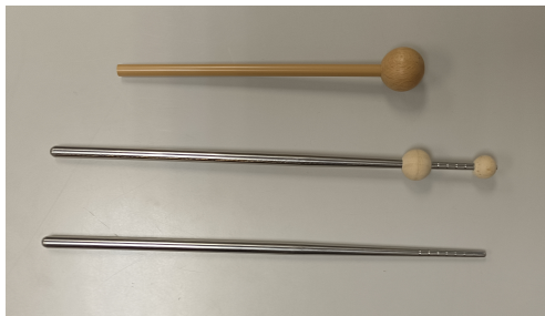
Figure 3: Mallets used for acoustic characterisation, from top to bottom: wooden mallet, metal mallet with shaped head and metal mallet.
