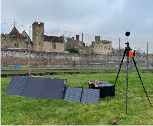
Figure 1: Field deployment configuration at the Penshurst site: the IMS NoiseGuard terminal and EcoFlow auxiliary power station within water-resistant enclosures, a 160 W solar array, and a Class 2 microphone tripod-mounted at 1.5 m over grass.
