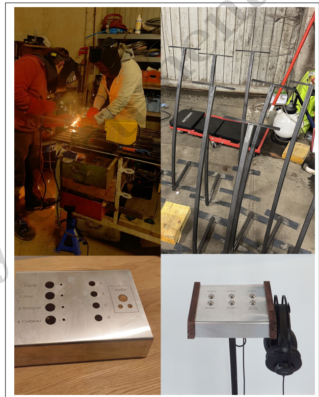
Figure 4: Top left: welding of module feet, top right: welded feet, bottom left: engraved and folded casing and bottom right: finished module.
