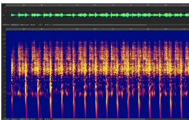
Figure 8. Spectrogram of a hand loom (22-second time segment) [Analysis: Beat Hohmann]
