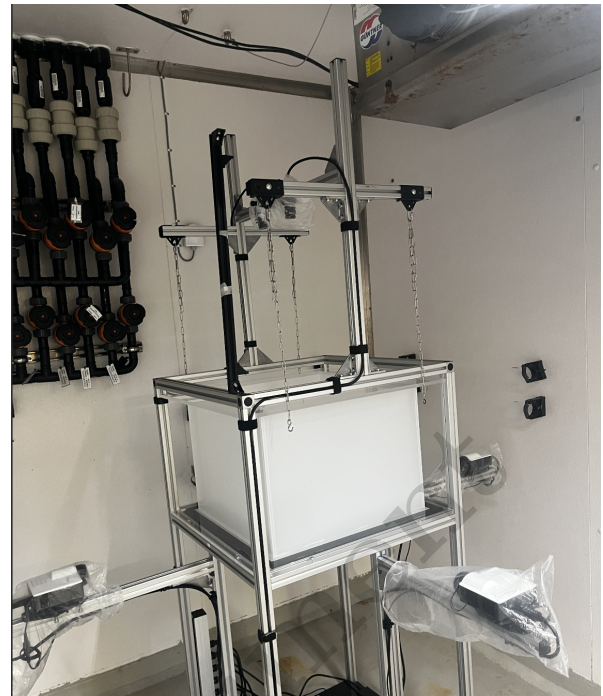
Figure 1: Experimental setup used for the automated acoustic measurements. The water tank is mounted within a rigid structural frame supporting a three-axis positioning system. The tank is mechanically suspended to reduce coupling with external vibrations, while the surrounding instrumentation enables synchronized signal playback and recording.
