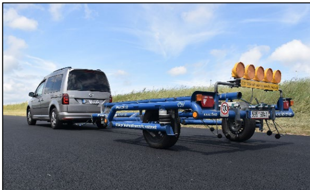
Figure 1. Open CPX trailer used for measurements (designed by CDV).
