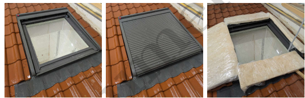
Figure 4: Roof window in the test stand — left: roller blind open; center: roller blind closed; right: frame area covered with soft insulation material
