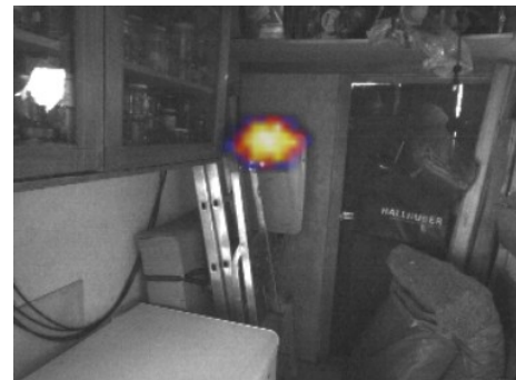
Figure 2. Localisation image produced by the acoustic camera.
