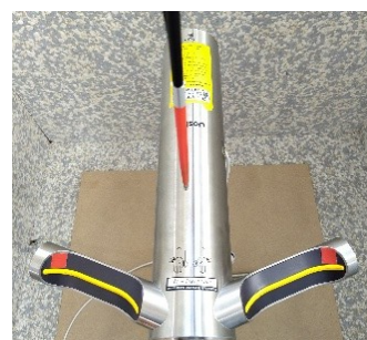
Figure 10. Dyson Airblade 9kJ hand dryer as installed within the scanning unit of the PTB.
