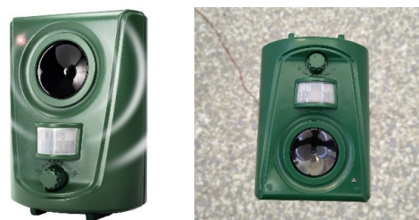
Figure 7. A photograph of the marten repellent tested (left), and the same device installed in the scanning unit at PTB (right).
