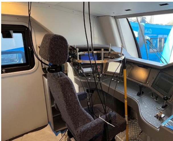
Figure 2. Measurement setup acc. to ISO 3381.
