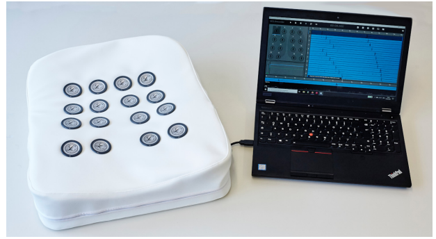
Figure 1: Sixteen-channel electronic stethoscope used for multi-channel lung sound acquisition in the clinical setting.
