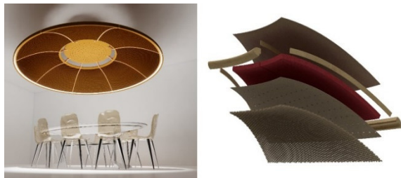
Figure 2. Design of a sound-absorbing system made of cardboard and other materials by Carmela Benevento e Cataldo Malena, created during the workshop.
