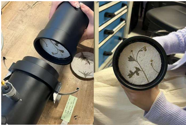
Figure 5. Installation of the sample in the impedance tube. (Source: by authors)
