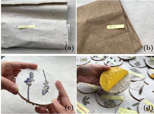
Figure 3. (a) Xuan paper from paper mulberry bark; (b) jute fabric; (c) bonded surface and acoustic layers; (d) double-sided tape applied to the back of the sample. (Source: by authors)
