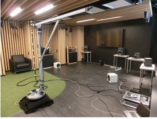
Figure 1: Photograph of the measurement room with the measurement robot and the loudspeakers.
