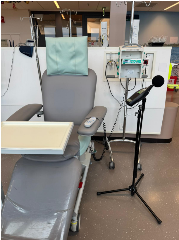
Figure 1: Typical in-situ measurement setup (Bruel and Kjaer 2250, tripod-mounted, windshield fitted). Measurements were conducted during daytime hours on weekdays across 20–30 locations per department.
