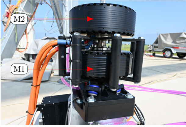
Figure 1: View of drive train consisting of two coupled Emrax 268 MV+42% connected by stator cage.
