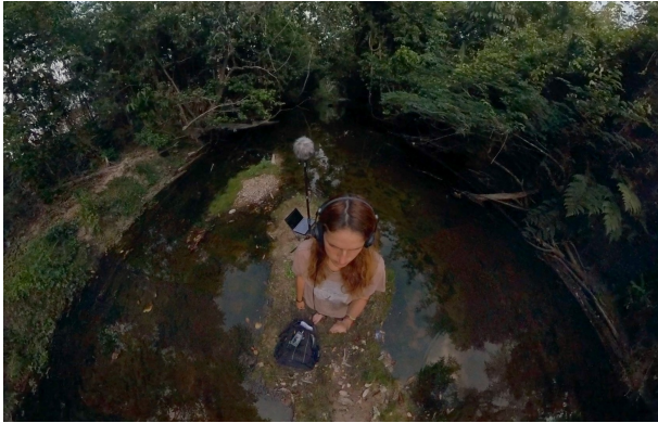
Figure 4: Field deployment at the Yguraman region (Measurement ID: YGURAMAN05). This image is an excerpt from the synchronized Insta360 video captured during the measurement. The setup demonstrates the spatial relationship between the HEAD acoustics SQobold binaural system (worn by the operator) and the Zylia ZM-1E Ambisonic array, positioned to capture the acoustic baseline of the riparian biotope.
