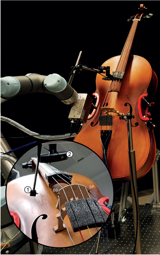
Figure 3: The setup: automated impact hammer (1), webcam (2) and two accelerometers (PCB Model 352C23) attached to the bridge at positions BB and SP.
