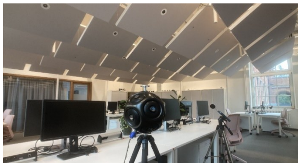
Figure 8. Configuration 4. with tilted ceiling panels from 3110-2500mm.
