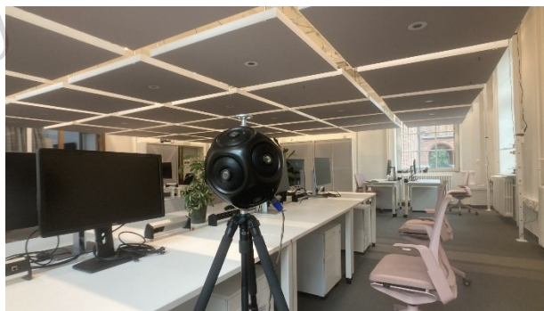
Figure 7. Configuration 3. with ceiling panels at 2100mm height
