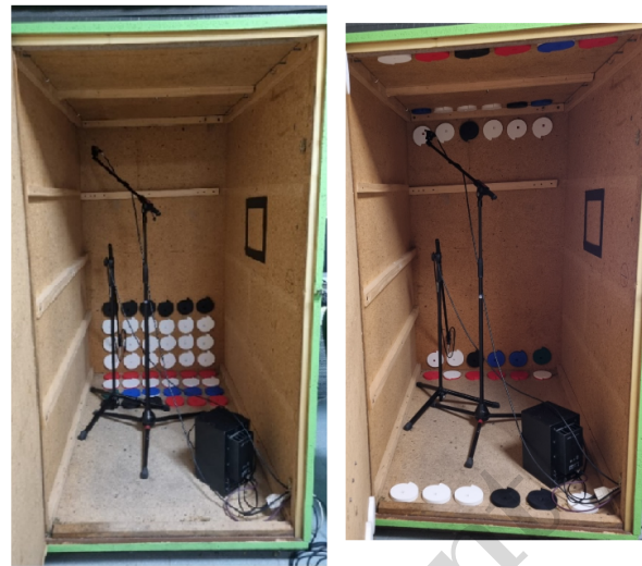
Figure 7: Distribution of the metasurface units inside the enclosure for evaluation of sound reduction. Left: 48 units placed on both sides of one short edge of the enclosure. Right: Two rows of 6 units are placed on both sides of each enclosure short edge.
