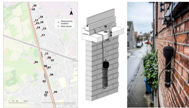
Figure 2. Locations of measurement points (left) and installation details (middle and right).
