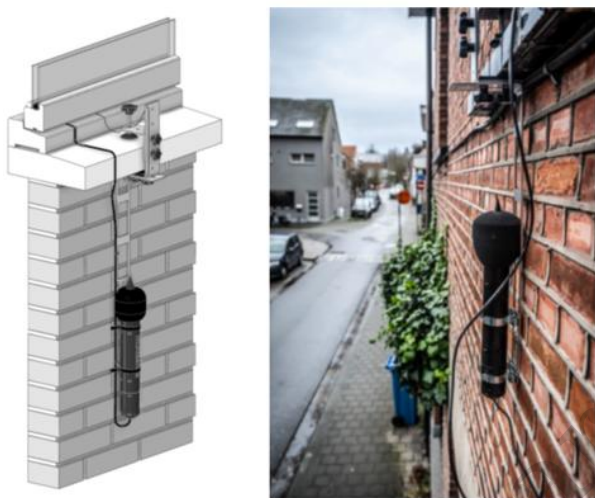
Figure 1. Installation of the Munisense smart sound sensor with custom-built mounting frame: (left) figure from the instruction manual and (right) actual installation by a citizen scientist.
