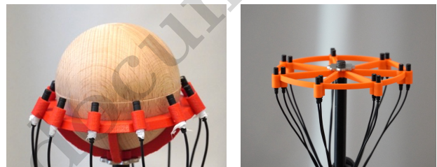
Figure 1: 5th-order EMA with pressure sensors and baffle, R = 40 mm (left), and 3rd-order EMA with virtual cardioid sensors and no baffle, R = 60 mm (right).
