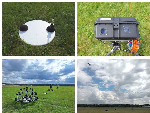
Figure 1: Measurement setup: INV and GND microphones for SPL calculation (top left), CAM for visual detection in case (top right), full sensor setup with ARR, SPL, CAM and METEO (bottom left), and level-flight of DJI FlyCart 30 with payload for MTOM (bottom right).
