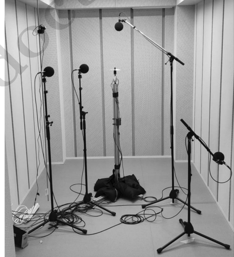
Figure 1. Aeroacoustic test bench for propeller design comparison.
