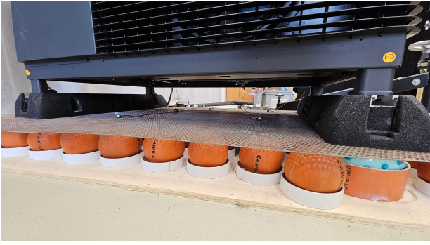
Figure 1: Heat pump A with rubber granulate mounting socket on the light reception plate, bearing of air-filled rubber balls.
