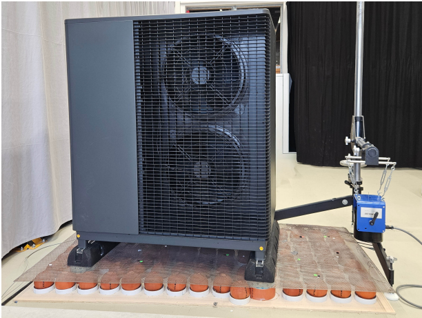
Figure 2: Heat pump A with rubber granulate mounting socket on the light reception plate.
