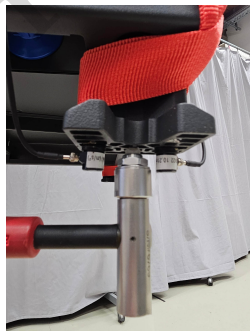
Figure 4: Setup for direct measurement of source mobility of the heat pump A.
