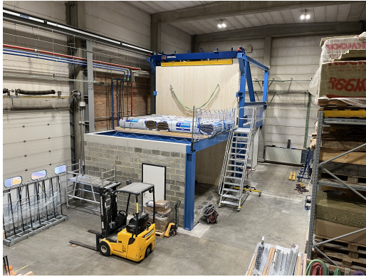
Figure 2: View of the CLT X-junction with floors covered with mineral wool packages.
