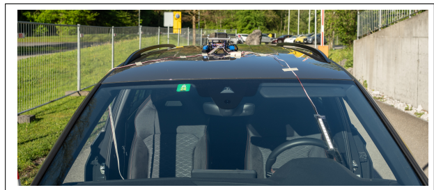
Figure 1: Module for measuring position, velocity and acceleration mounted on a test vehicle. Acceleration indicator LEDs are on the windshield for real-time feedback.
