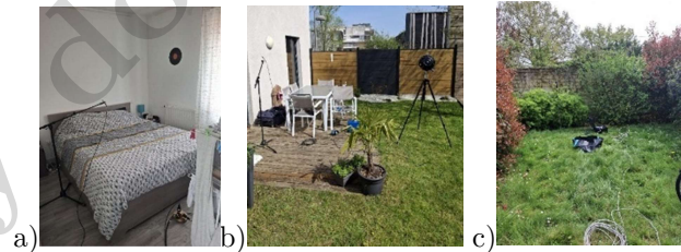
Figure 2. Photos of the test setup for the acoustic and vibrational characterization of the site, a) Instrumentation of a participant's room, b) Microphone on the facade and noise source used for air-borne transfers; c) measurement station at the property boundary, closest to the source (railway network).
