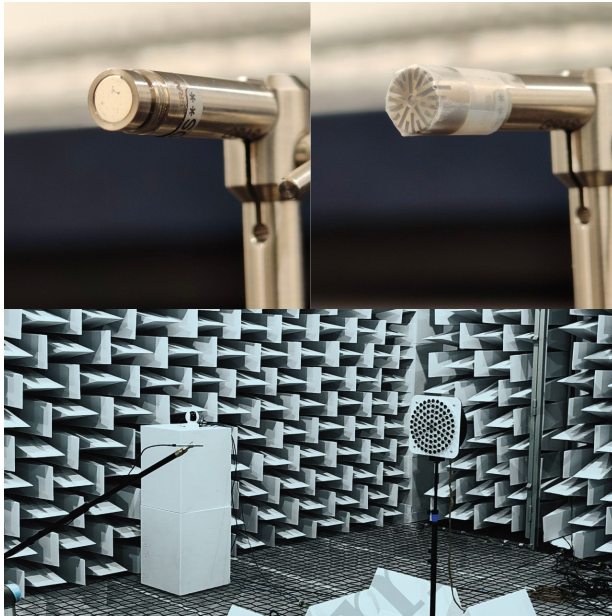
Figure 1: Top row: 1/4" microphone without grid (left) and with acetate tape (right). Bottom row: experimental setup, with UR5 robot and the analysed PAL.
