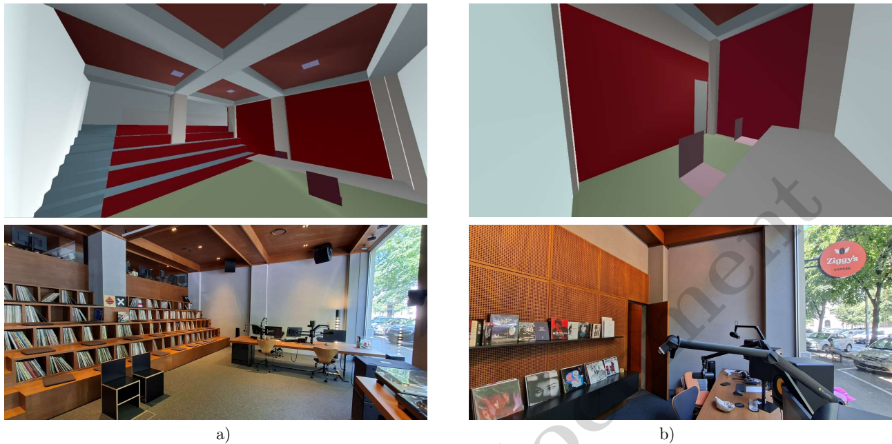
Figure 3. Three-dimensional acoustic models developed in ODEON (top) and the corresponding finished spaces (bottom): (a) Studio 1; (b) Studio 3.
