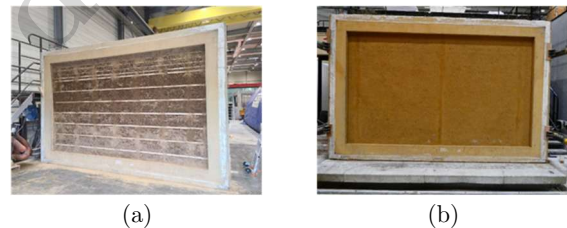
Figure 7. Light earth wall tested: (a) bare, (b) coated both sides.
