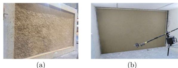
Figure 8. Wattle and daub wall tested: (a) bare, (b) coated both sides.
