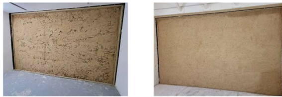
Figure 2. Two faces of the bare cob wall tested.
