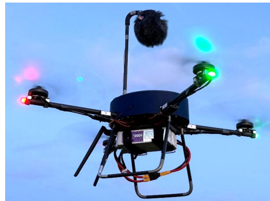
Figure 2. Modular quadcopter with on-board noise measurement.
