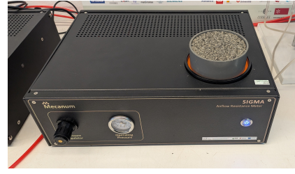
Figure 3: Airflow resistivity ( \sigma ) testing machine with sample.
