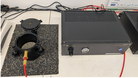
Figure 2: Open porosity ( \phi ) testing machine with sample.
