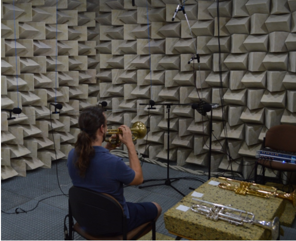
Figure 3: Experimental setup and player in the recording position.
