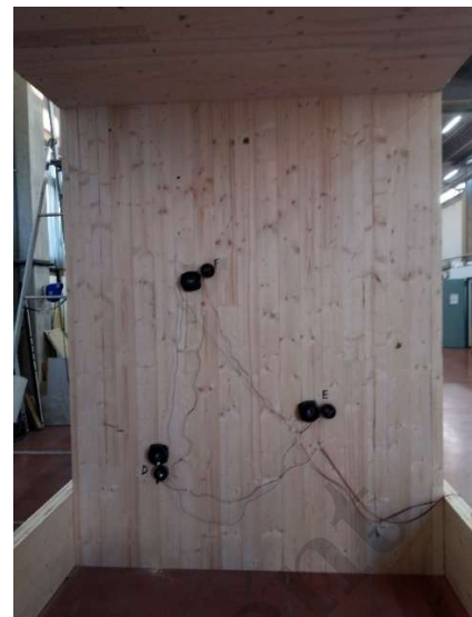
Figure 1. Horizontal X-junction mock-up in CLT (left). Three pairs of vibroacoustic transducers in three source positions (right).
