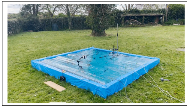
Figure 1: Water basin set up showing the source loud-speaker, microphones, ripple height probes and ripple generator.
