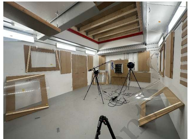
Figure 2. Source room with a lightweight deck in the test opening, showing semi-frustum of a cone diffusers, surface diffusers, tuned absorbers and measurement equipment.
