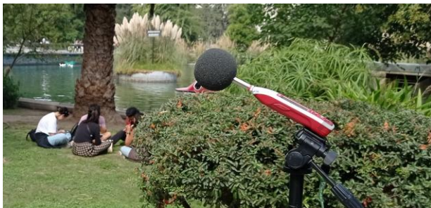
Figure 2. Sound-level measurement and participant surveys during field data collection in Quinta Normal Park, Santiago, Chile.
