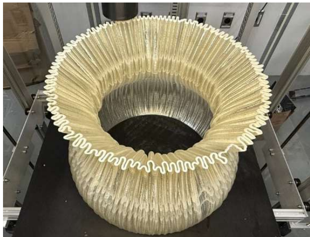
Figure 6. Pellet-based extrusion fabrication of a Harmonic Artifact 9 using a Gigabot additive manufacturing system.
