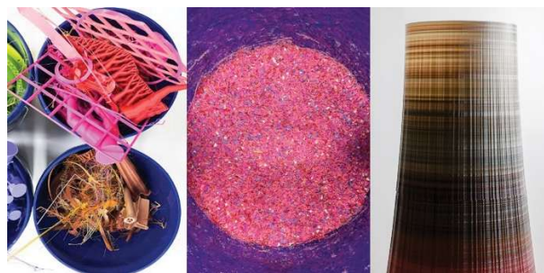
Figure 8. Circular PLA workflow from discarded prints (Left) to recycled feedstock (Center) and pellet-based extrusion fabrication (Right) of a harmonic artifact on a Gigabot system.
