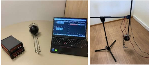
Figure 3. In-situ impedance measurement setup
