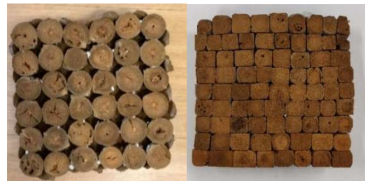
Figure 2. Bonded oak-apple panel specimens: Sample A (left), assembled from halved oak apples, and Sample B (right), assembled from machined cuboid elements
